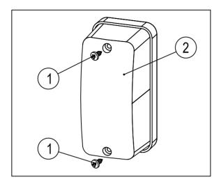
The taillights are LEDs, it not working use a replacement tail lamp assy.
