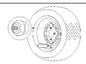
Rear Tapered nuts: install with tapered side against wheel.
