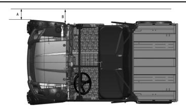
The recommended toe alignment is 1/8" to 1/4"(3 to 6mm) toe out.
