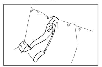
Recommended lubricant: Lithium-soap-based grease (all-purpose grease)
